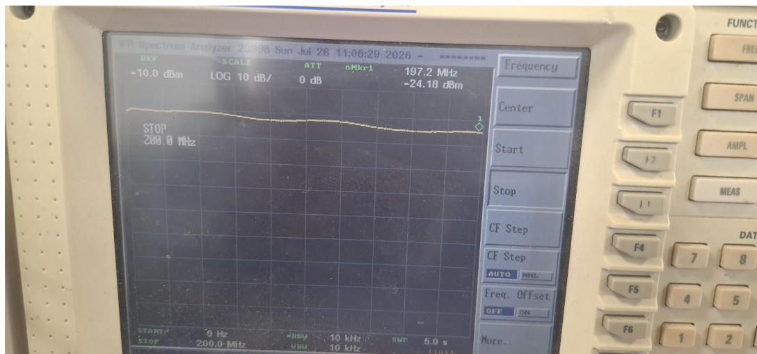
Figure 2. Non-selected channel measurement showing isolation of more than 60 dB; a second channel (not shown) exceeded 70 dB.
