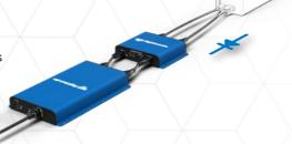
The Neous isolation core implements HW enforced unidirectional data flow and encrypts/decrypts the HID data.
