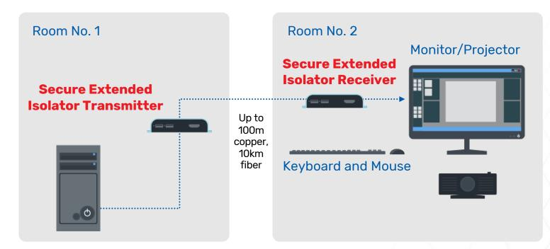
The HSL Secure Extended Isolators remotely transfer not only video and audio, but also the keyboard and mouse. The remote PC can be securely operated from the monitor/projector side. The Keyboard/Mouse USBs are unidirectional, filtered and secure.
