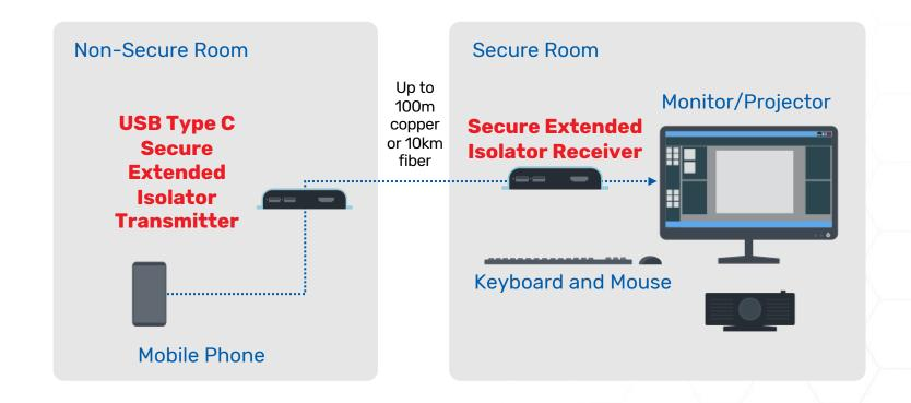
The Secure Extended Isolator with a USB Type-C port provides a secure connection to the phone that is left outside the secure room, without compromising the security of other devices in the secure room.
