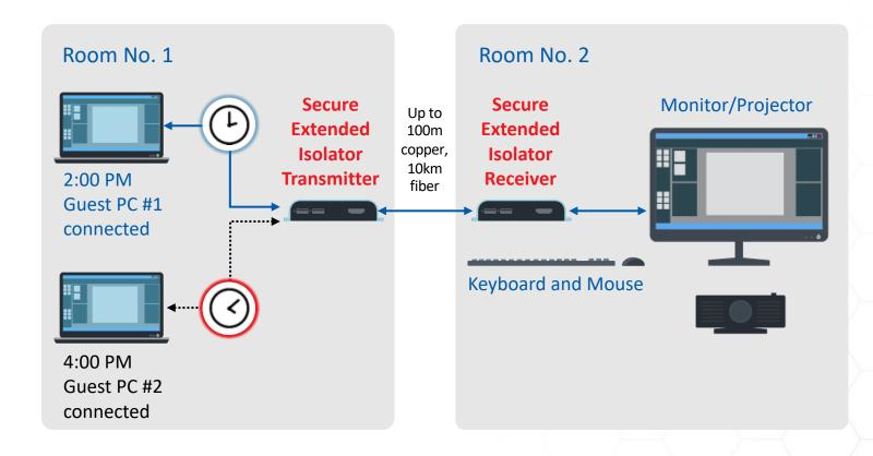
Problem solved (above) by connecting an isolator between the computer and the display/KBD/mouse, preventing data leakage between the computers.
