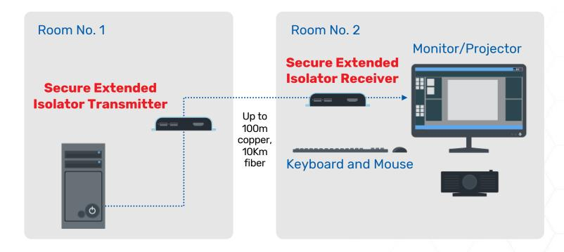
The HSL Secure Extended Isolators have the KVM ability to remotely transfer not only video and audio, but also the keyboard and mouse. The remote PC can be securely operated from the monitor/projector side. The Keyboard/Mouse USBs are also unidirectional and secure.
