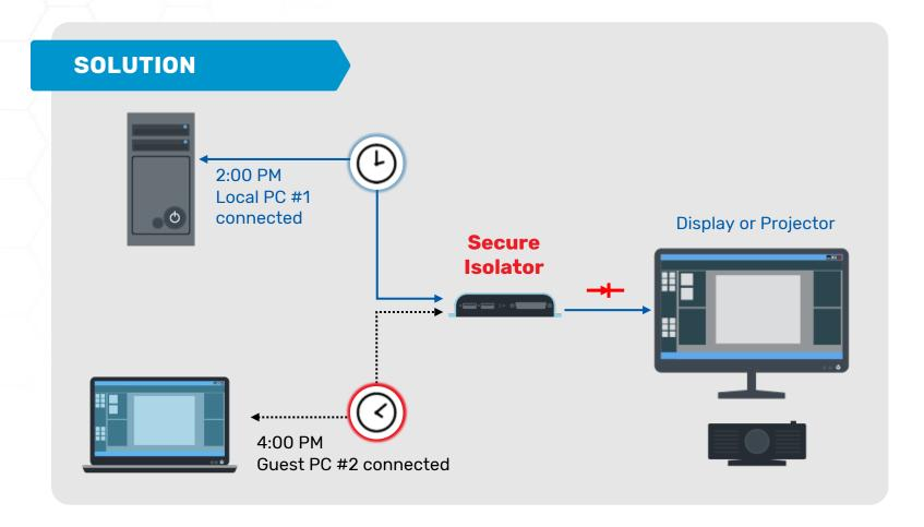
Problem solved by connecting an Isolator on the cable between the computer and the display, preventing data transfer from the display to the guest computer.
