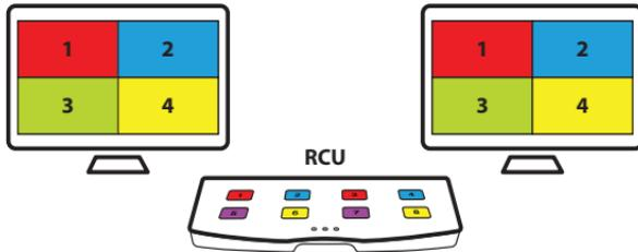
3. 8-port Matrix: Buttons 1-8 switch Channels 1-8 on the left display.
