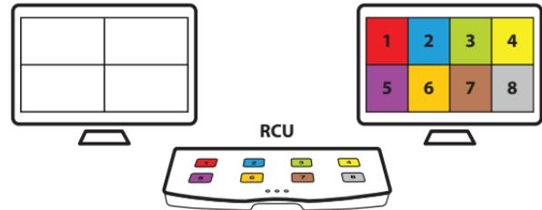
5. KVM Combiner: Buttons 1-4 switch Channel 1-4, Buttons 5-8 switch Channel Presets 1-4.
