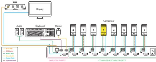
**Figure 3:** RCU connected to an 8-Port KVM Switch
