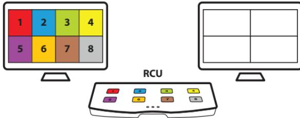
4. 8-port Matrix: Buttons 1-8 switch Channels 1-8 on the right display.
