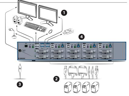
audio-out ports using an audio cable. Connect one end of the cable to the computer's audio port using the 1/8" (3.5mm) stereo plug. Connect the other end of the audio cable to the KVM audio-in/audio-out computer port.
