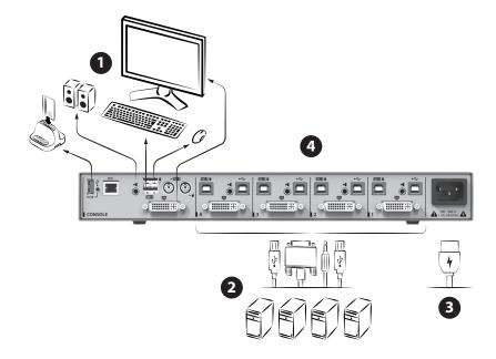
1/8" (3.5mm) stereo plug. Connect the other end of the audio cable to the KVM audio-in computer port.
